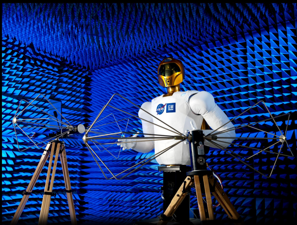
Robonaut 2 Undergoing EMI Testing
